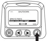
The Single or Four parameter screen will display the fault icon until the fault condition is corrected. NOTE: Ignoring active fault codes could result in severe engine damage.
